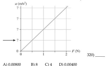
321) The figure shows an object's acceleration-versus-force graph. What is the mass of this object?
