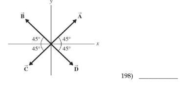
199) The figure shows four vectors,  $\vec{A}$ ,  $\vec{B}$ ,  $\vec{C}$ , and  $\vec{D}$ . Vectors  $\vec{A}$  and  $\vec{B}$  both have a magnitude of 7.0 cm, and vectors  $\vec{C}$  and  $\vec{D}$  both have a magnitude of 4.0 cm. Find the magnitude and direction of the sum of these four vectors.
