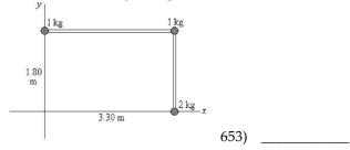
654) The L-shaped object shown in the figure consists of three small masses connected by thin uniform rods, each rod of mass 3.00 kg. Assume that the masses shown are accurate to three significant figures. How much work must be done to accelerate the object from rest to an angular speed of 3.25 rad/s about the *y*-axis?
