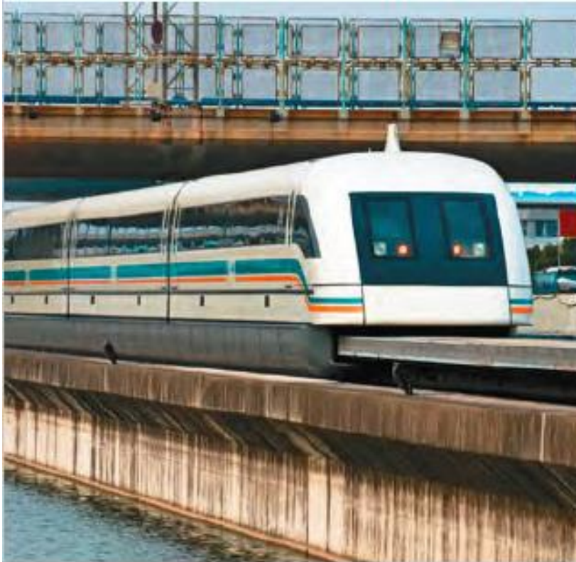
▲ FIGURE 19.6 A maglev train in Shanghai. Maglev (“magnetic-levitation”) trains use superconducting electromagnets to create magnetic fields strong enough to levitate a train off the tracks.
