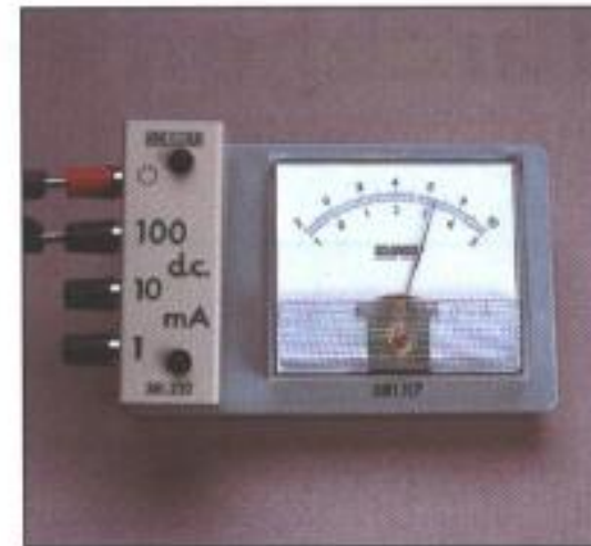
Figure 3.6 An ammeter fitted with a shunt.
