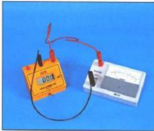
Figure 3.4 First set up the circuit and decide where you wish to measure the current. Then break the circuit at the required point.
