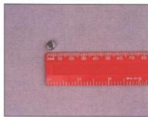
Figure 2.6 A bearing-aid battery will supply 10\ \mu\text{A} continuously for 6 months
