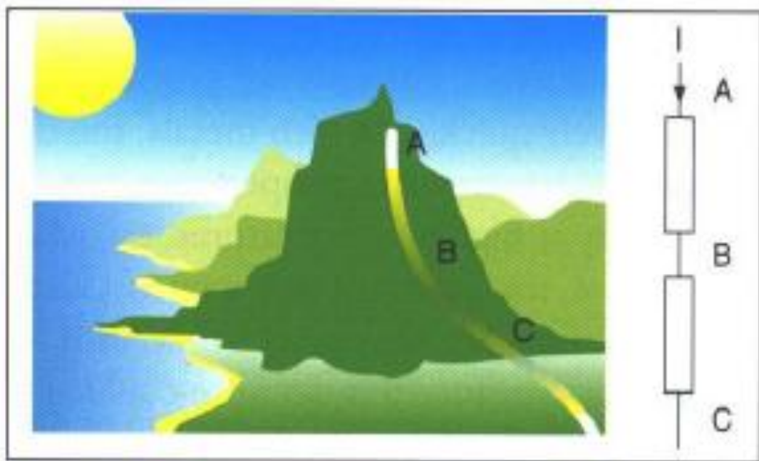
Figure 14.6 Current flows through a chain of resistors like water through a channel
