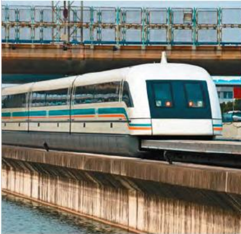
▲ FIGURE 19.6 A maglev train in Shanghai. Maglev (“magnetic-levitation”) trains use superconducting electromagnets to create magnetic fields strong enough to levitate a train off the tracks.
