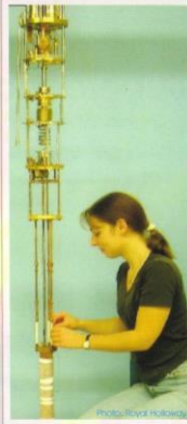
Ultra low temperature cryostat used for experiments on superfluids down to 100 \mu K.
