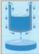
A beaker of superfluid empties spontaneously as the liquid flows over the side through the moving film.
