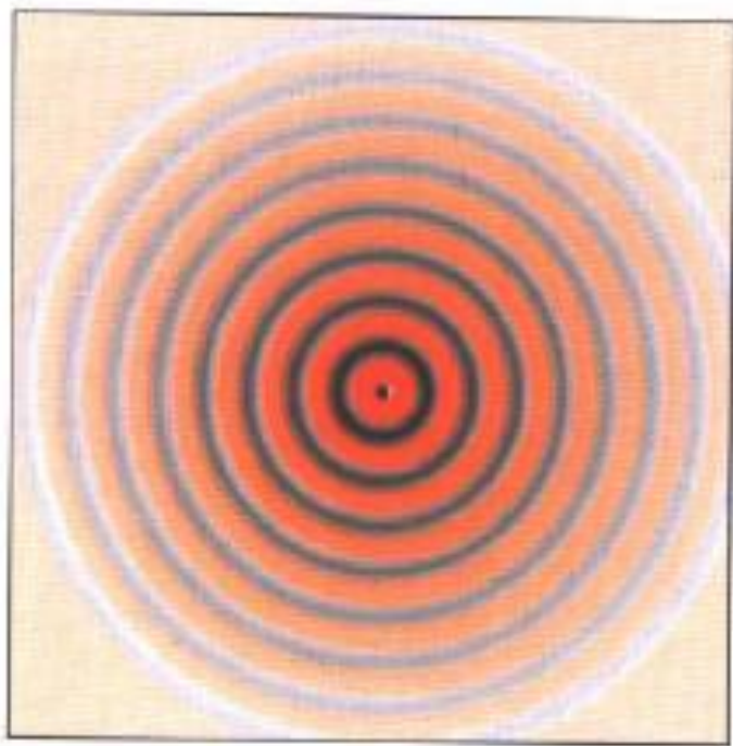
Figure 23.4 The superposition pattern for many gratings at different angles
